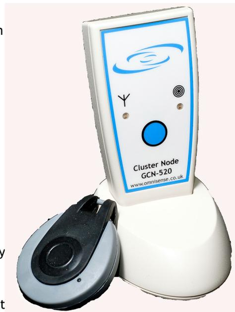
The Series 500 products are based on 802.15.4 and 802.15.4a radios which are compatible with Wireless Networking standards adopted by the Continua Alliance. This potentially allows the system to interface to other wireless healthcare devices in the future.
