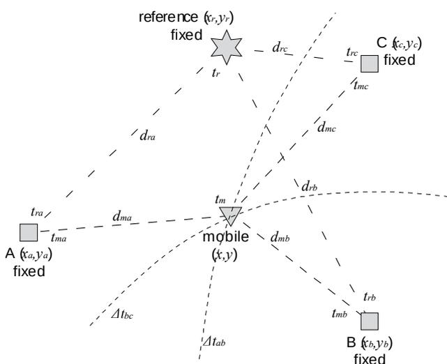
Such systems sometimes operate in an “inverted” mode in which the tag measures signals transmitted periodically by the Fixed Receivers - as, for example, in cellular mobile systems using OTDOA.
