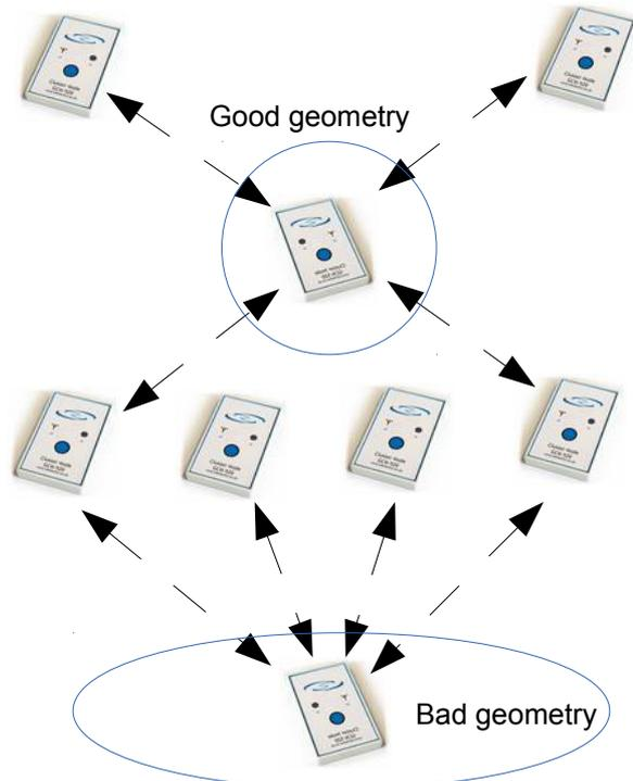
The issue of geometry is particularly important to consider when configuring fixed devices and for situations in which operation at or near the edges of the network is required. It is good practice, where possible, to ensure that there are enough fixed devices installed around the periphery of the operating area so that mobiles are always surrounded by fixed nodes.
