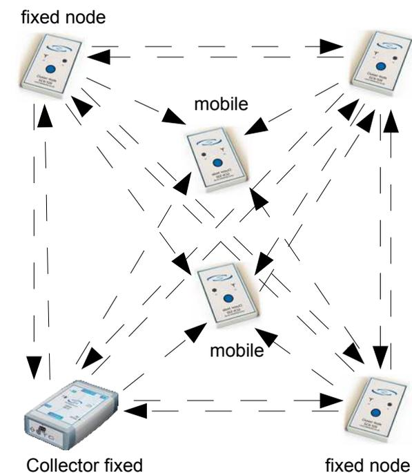
In this example the fixed nodes operate fully meshed with one another, but the mobiles only receive chirps and don't transmit.
